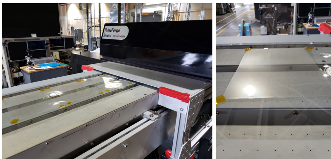
Figure S12. R2R photonic curing tool: Images of hybrid TCEs just after being conveyed through the R2R photonic curing tool. The flash lamp is enclosed in the black box, labeled PulseForge Invent, in the left image.
