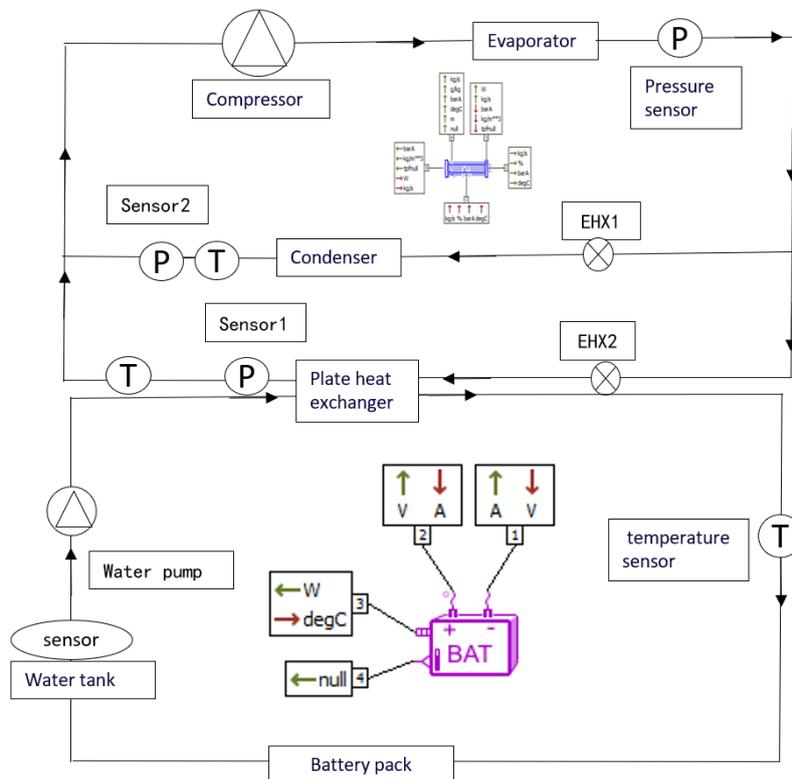
**Figure 1.** Schematic diagram of the heat pump system..
