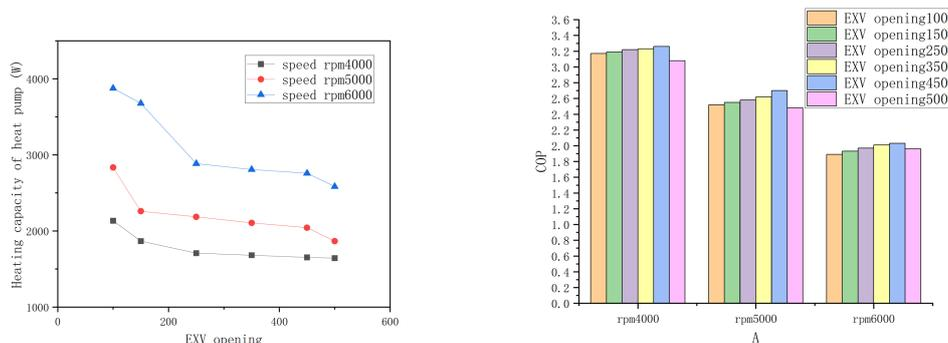
**Figure 4.** Heating capacity and COP at different EXV openings..
