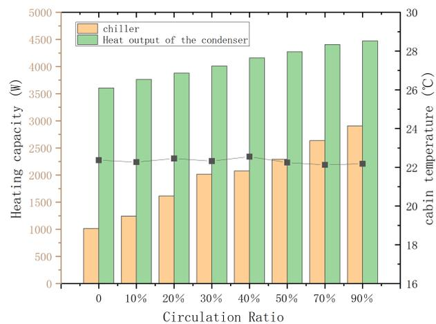
**Figure 5.** Heating capacity of heat pump systems under different heating cycle ratios..
