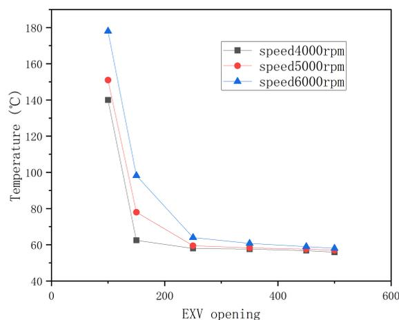
**Figure 3.** Impact of Different Expansion Valve Openings on Exhaust Performance..
