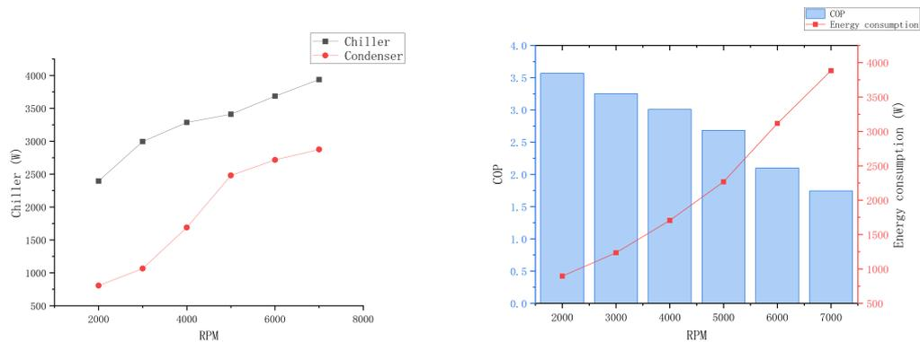
**Figure 6.** Cooling Capacity and COP of the Heat Pump System at Different Compressor Speeds..
