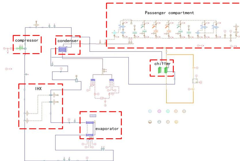
**Figure 2.** One-dimensional model for heat pump air conditioner heating..
